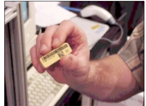
Using a self-contained laser system, Boeing generated bar-code labels like this one for Chinook components to facilitate parts tracking and inventory management.
