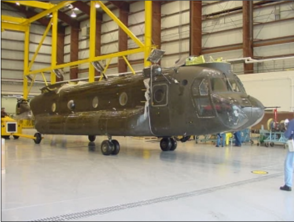
The Chinook Composite Maintenance Trainer allows helo users and maintainers to perform and practice most of the maintenance duties they will encounter with the aircraft they purchase.
