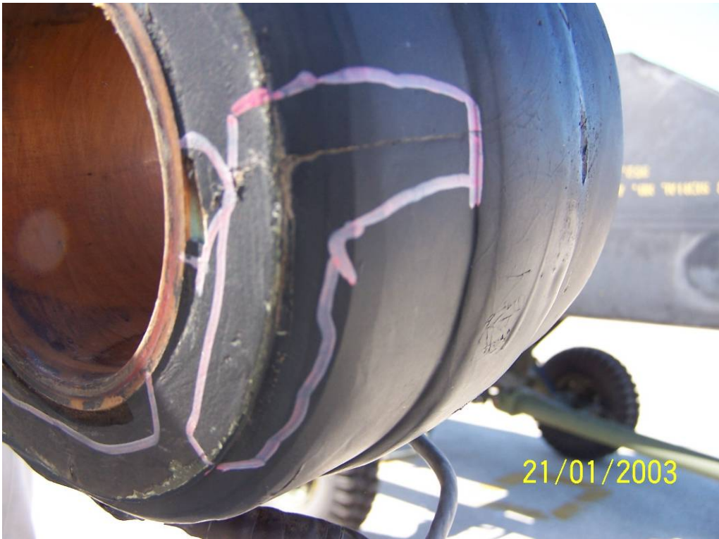
Figure 12, Example of Suspect Indication & Cracked Pad
