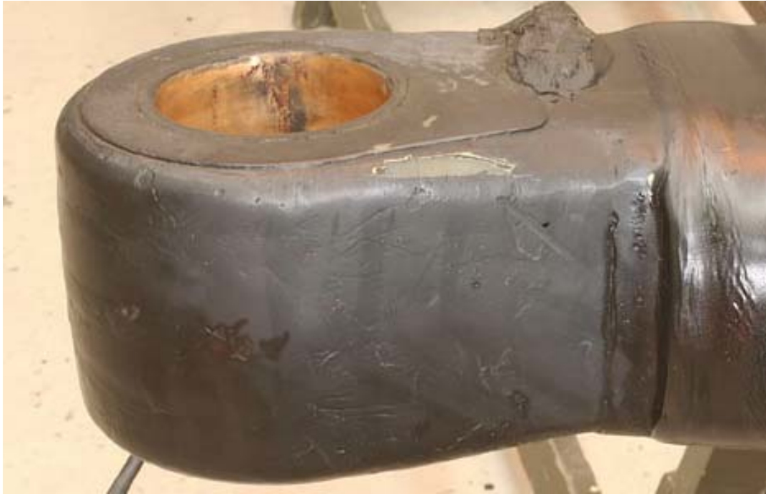
Figure 10, Example of a Sanded Root End Crack
