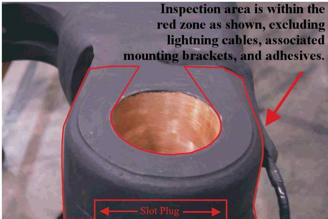
Figure 6, Off-Aircraft Inspection Area
