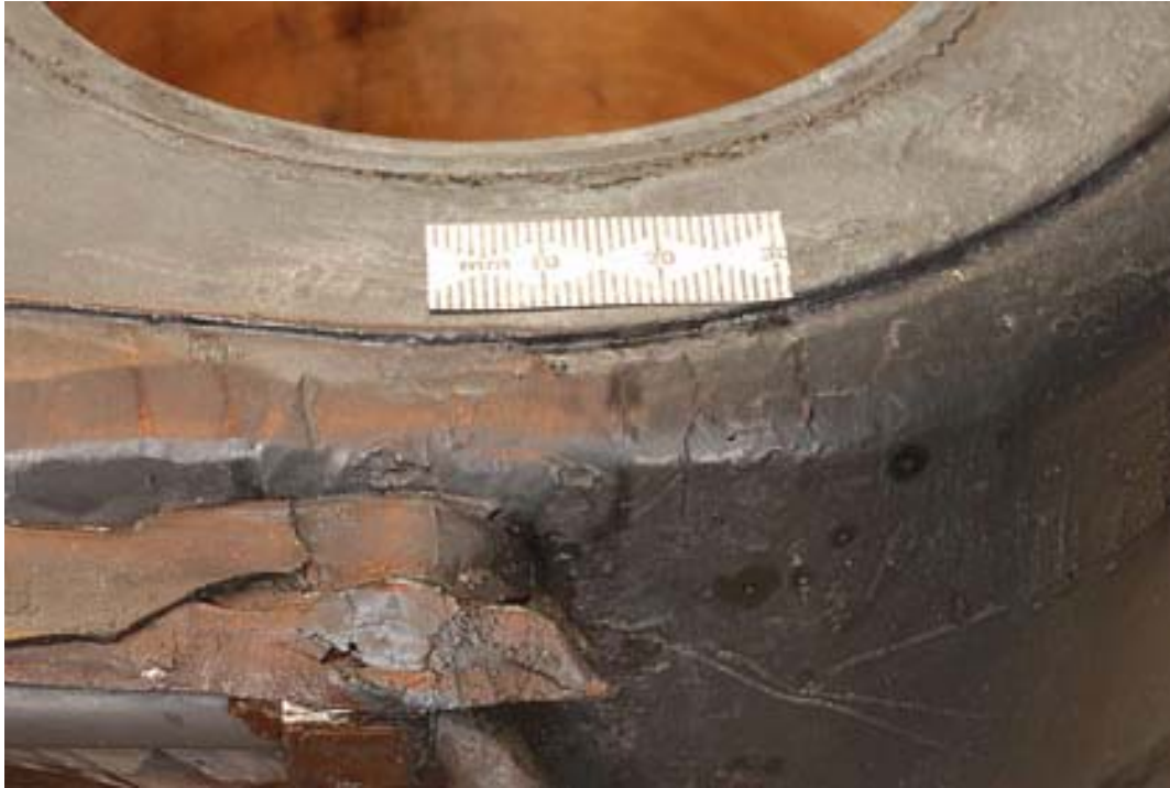
Figure 8, Example of an Un-sanded Root End Crack
