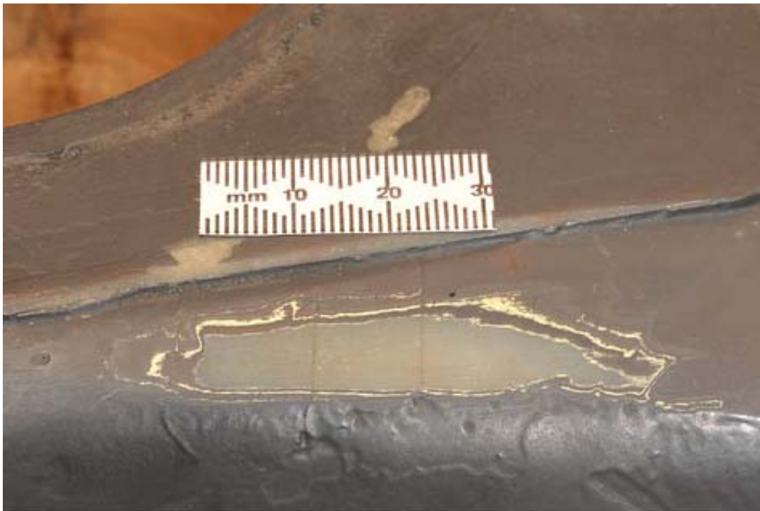
Figure 11, Example of a Sanded Root End Crack
