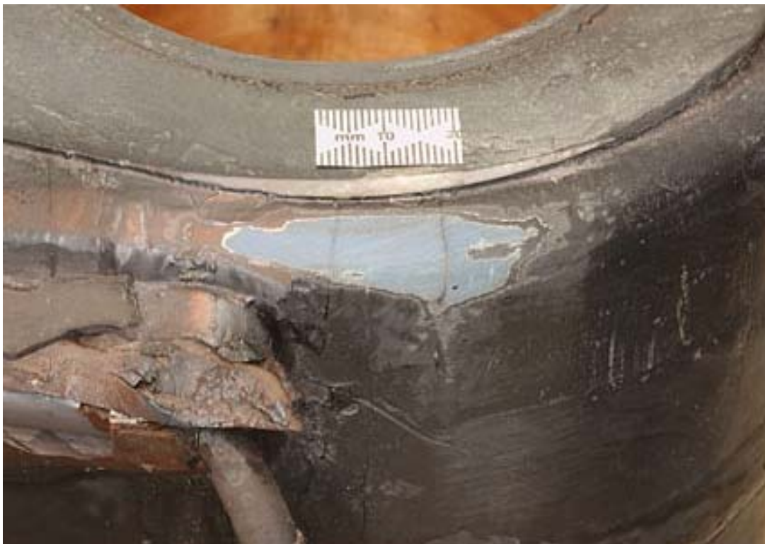
Figure 9, Example of a Sanded Root End Crack
