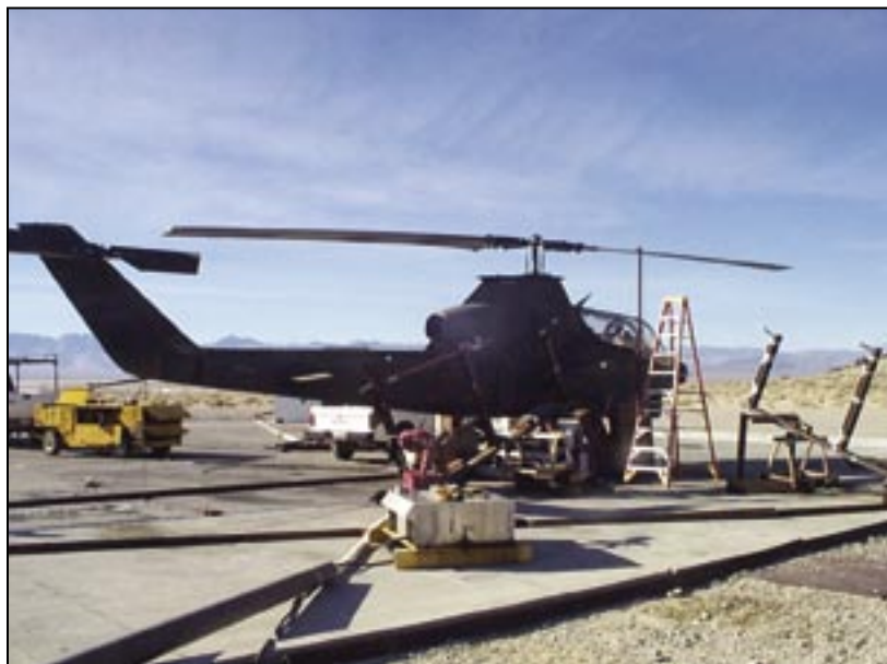
Figure 6. Near-miss test setup, shot 6
