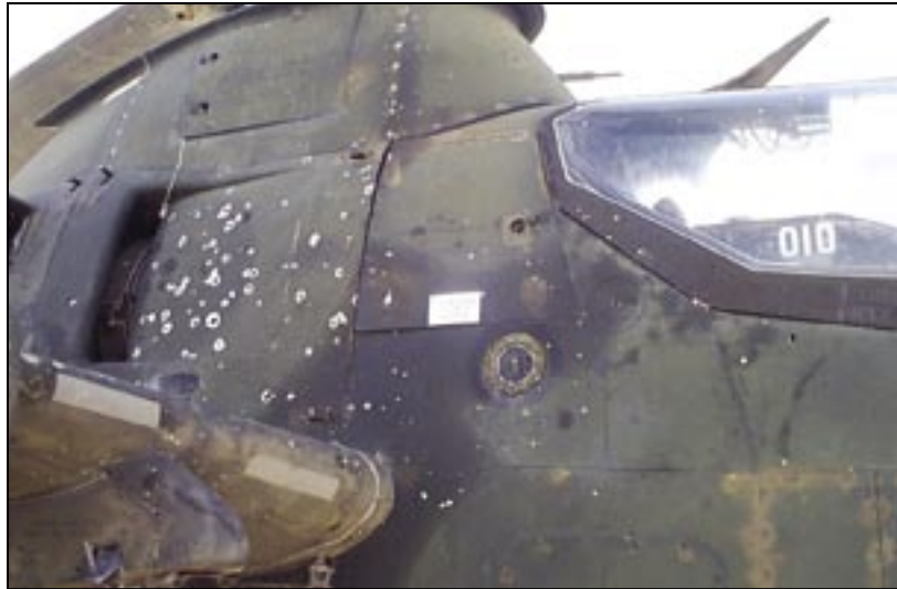
Figure 5. Fragment damage to access doors, skin, and cockpit canopy, shot 6
