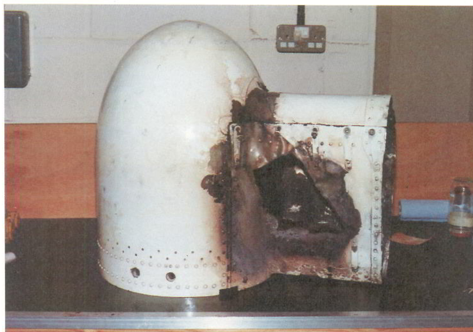
(ii) Fire damage: No 1 engine transmission gearbox fairing
