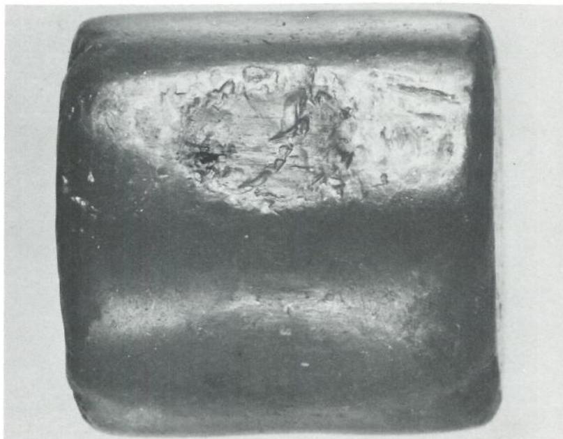
(iii) Typical example of roller damage
